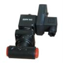
3GD series utilize timer based drain valve. The condensate is collected in a chamber is segregated from the air flow. The drain valve starts operating automatically after 4/16 mins and opens 4/8 secs for draining, depending upon the capacity of the dryer
