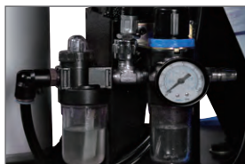
Pressure limiter, air filter and oil reservoir for lubricant to ensure the safe operation and durability of the machines
