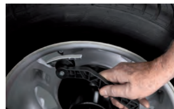
Gauge arm equipped with weight clamp retains the wheel weight in the correct position for weight placement
