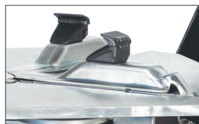
Tried, tested and proven clamps with plastic protection on existing machines are used
