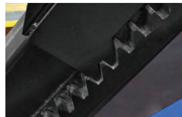
15 level locking positions with pneumatic lock release system
