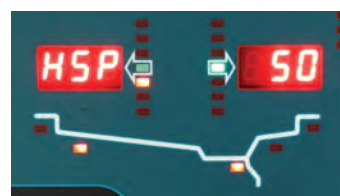
Easy identification of ALU mode with bright LEDs indicating selected weight position
